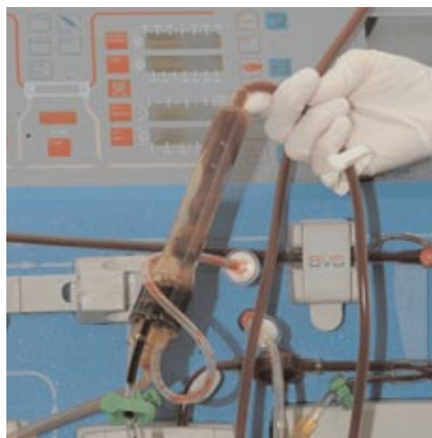
Fig. 1B. Clotting in the venous bubble trap inducing stop in dialysis in a patient at the end of a 4 hour hemodialysis session. The patient lost the blood volume in the filter and lines (about 200 ml).
