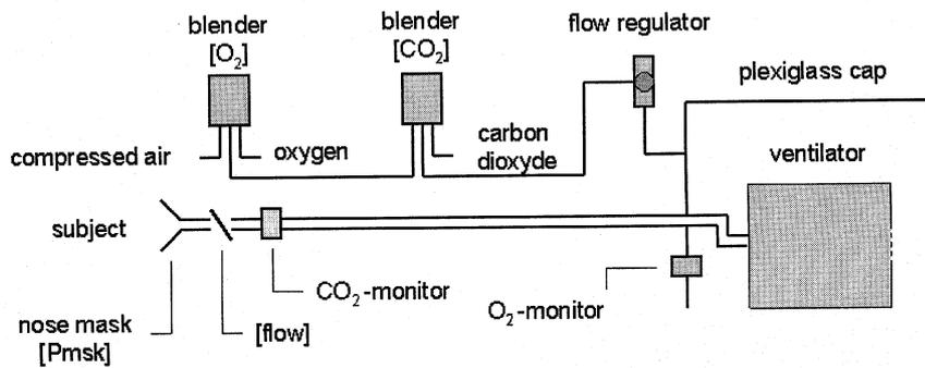
Fig. 1. Schematic diagram of the experimental setting. The ventilator is positioned under a plastic cap, where a constant milieu of carbon dioxide (CO<sub>2</sub>)-enriched air is provided by means of blenders for oxygen (O<sub>2</sub>) and CO<sub>2</sub>. Gas composition is controlled by an oxymeter (O<sub>2</sub> monitor) and a capnograph (CO<sub>2</sub> monitor). See text for further details.
